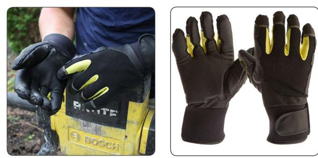
The IMPACTO AVPRO reduces vibration energy transmission to the palm, fingers and thumb. To designate a glove as Anti-Vibration per ISO 10819 standard, TRM medium frequencies must be less than < 0.90 and TRH high frequencies must be less than < 0.60. AVPRO -> TRM = 0.871 and TRH = 0.542. The AVPRO is in conformance with International Anti-Vibration Glove Standard ISO 10819:2003 Mechanical Vibration and Shock - Hand-Arm Vibration and North American Standard ANSI S2.73-2002 (R 2007).
