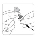
To attach cord, form a loop, position around groove at handle.
